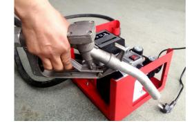
2. Connect on Power, pulse-on Motor.
