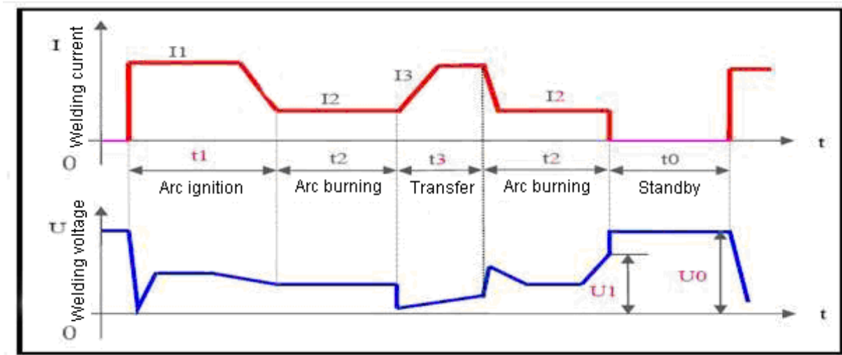
Fig 10.12 Current and Voltage Change during MMA
